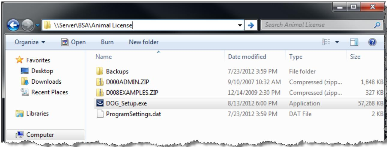
If the program version date is newer than the date of the program's executable on the server, the executable from the local workstation will be copied to the Shared Program Folder on the network and overwrite the existing executable.
